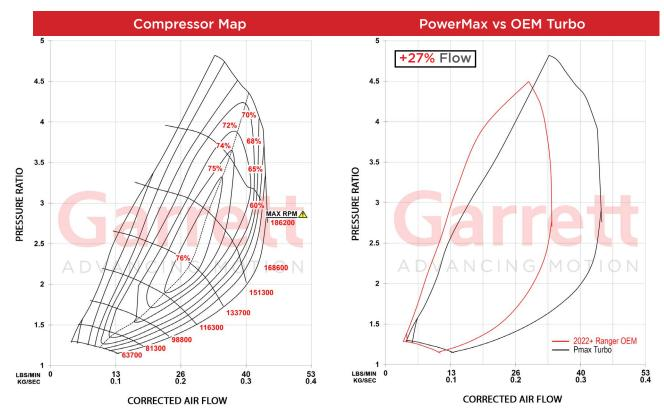
WARNING: Maximum allowable turbocharger speed is 186krpm. The use of this product above max turbocharger speed is at the owner's risk, and can result in damage and premature failure. To protect the turbocharger from overspeed when operating, a speed sensor can be installed into the compressor housing to monitor shaft speed. Sensors sold separately.
