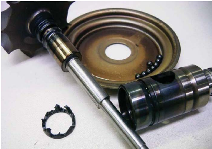
Overheated ball bearing cartridge, disassembled showing damaged retainer at lower left. Bearing races are blued and damaged as well. Excessive play is the result of retainer and race damage, often culminating in wheel to-housing rubbing and total turbo failure.
