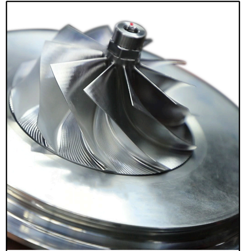
Fig C: Forged fully-machined 10 blade compressor wheel with G Series aero. G42-1200 flows 109 lbs/min 1200HP. G42-1450 flows 131 lbs/min 1450HP.
