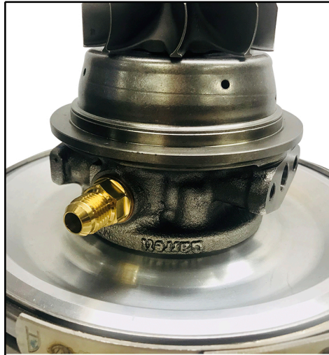
Fig B: New turbine aero has a peak efficiency of 77% and flows 10% more than GTX42. Aluminum backplate helps reduce weight. -6an water fittings come installed.
